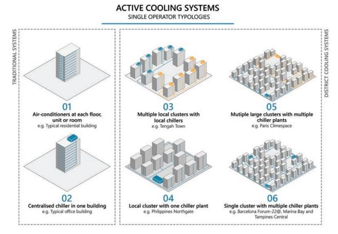
Figure 1. Typologies of active cooling systems. Image: Centre for Liveable Cities
