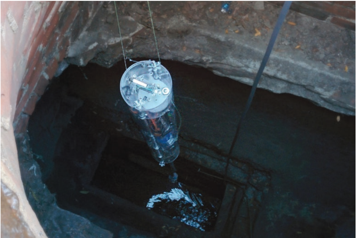
Robots designed by MIT Senseable City Lab to collect wastewater samples from the sewers. Image: MIT Senseable City Lab and Alm Lab
