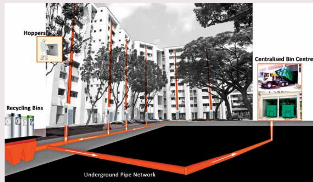
This diagram illustrates how the Pneumatic Waste Conveyance System transports household waste from each refuse chute to a centralised bin centre via a network of underground pipes.
